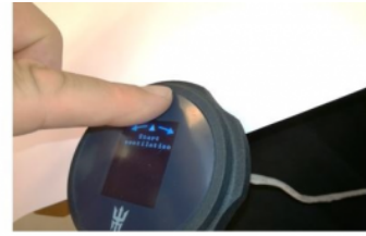
Step 5: Connect cable into heater. Start using :- rotate wheel -select by pressing top of panel
